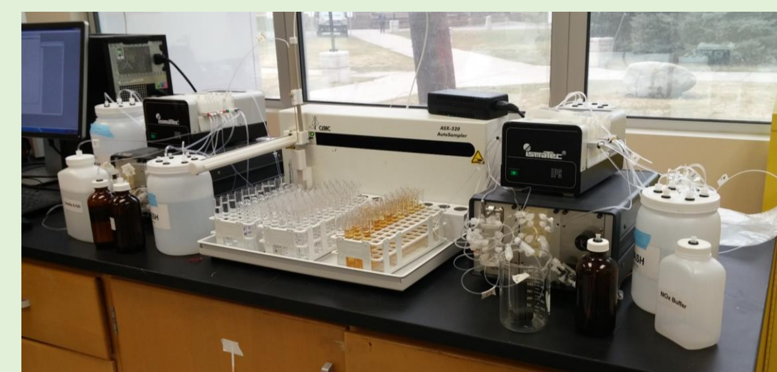
Figure 6: Alpkem 3 flow analyzer used to analyze water samples
