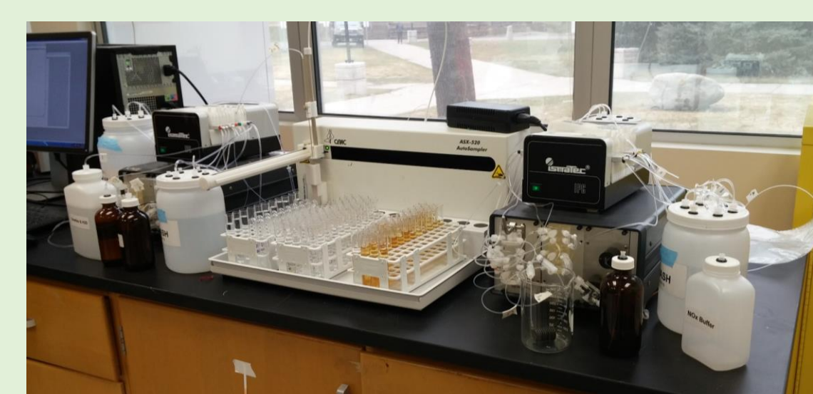
Figure 6: Alpkem 3 flow analyzer used to analyze water samples
