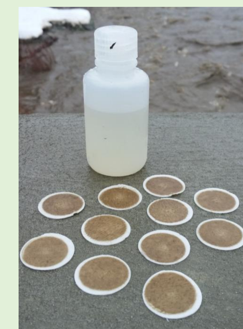
Figure 5: To collect less than 50 mL of filtered water, 11 filters were needed
