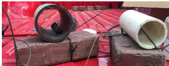
Figure 2. Temperature logger housing for placement in creeks.
